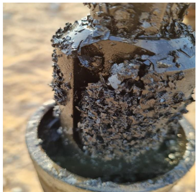
Feb 2021: Plunger stuck inside barrel due to scale
